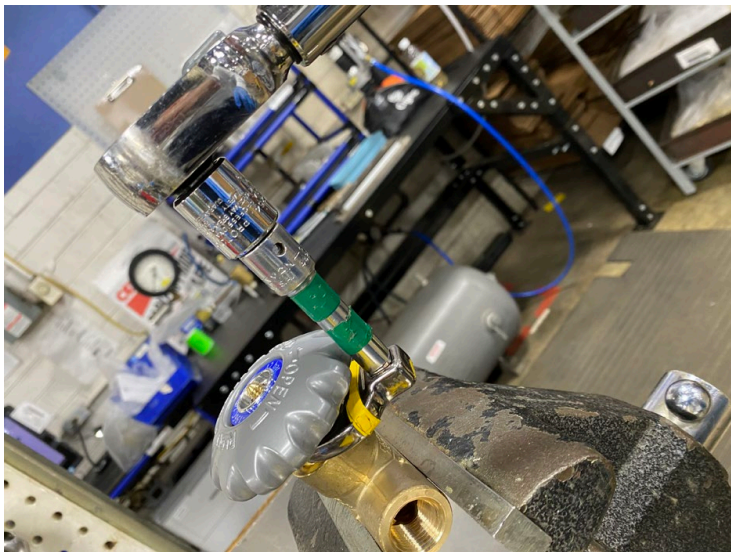
Figure 2: Final adjustment with torque wrench.
